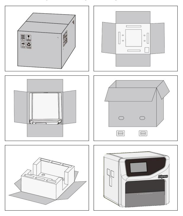
Figure 2-1. ZiXpress 96 Dx System - Instrument Unpacking
