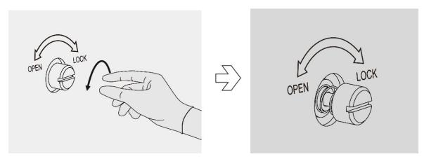
Figure 2-2. ZiXpress 96 Dx System - Open Transport Lock
