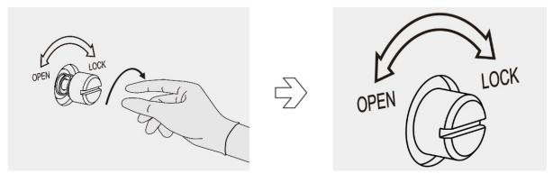
Figure 4-3. Lock Transport Lock
